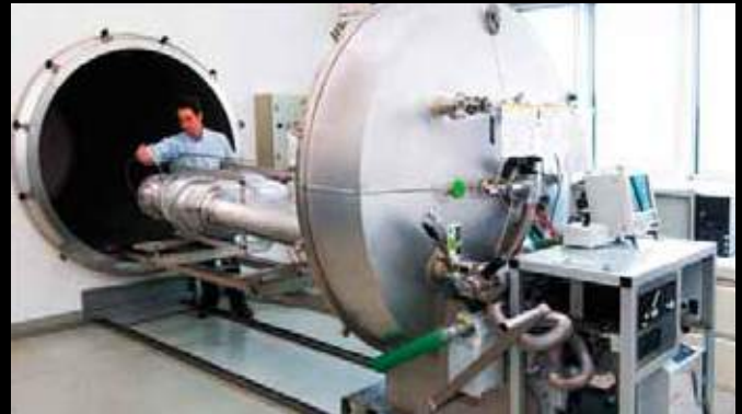
Integral test in vacuum chamber
